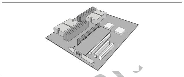
Figure 4-9. Assembled QHT7140 with Riser
